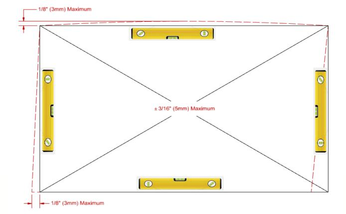
2. Make sure the frame header is designed to withstand the dead loads of all doors including glass plus momentum and impact loading since it is a top-hung door system. Rough opening header must not deflect more than 1/8" (2 mm) when carrying the weight of the doors according to hardware suppliers' specifications.
